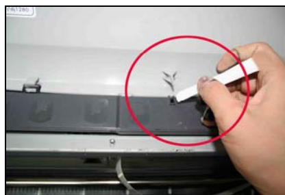
During using, pls keep the printer top cover opened. Insert the roll into the hole as in the picture.
