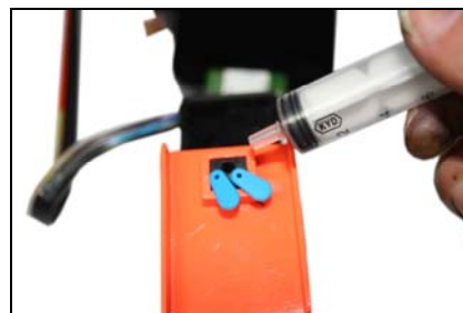
Insert the syringe into the opened hole.
