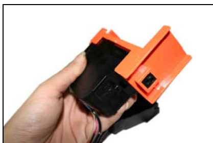
Cover the cartridge inside the HP refill tool as in the picture.
