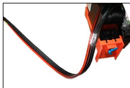
Vacuum the air of the other colors in the same way. After that, there will be no air inside the tube.
